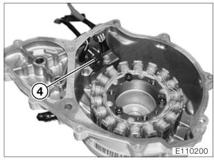
• If necessary, remove ignition trigger (4).
