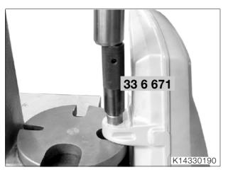
• Press in needle roller bearing with drift, **BMW No. 33 6 671**.
