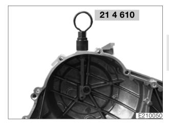
Using puller, BMW No. 21 4 610, pull out both • needle roller bearings and the sealing ring together.
