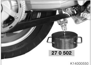
• Suspend weight, **BMW No. 27 0 502**, from the measuring device.
