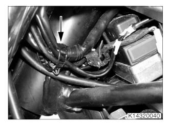
• Disengage the cable tie at the frame head (arrow).
